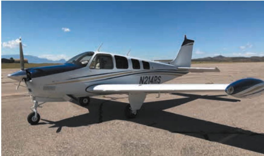
That's Ralph Scargall's 1977 A36 with 20-gallon tip tanks and the IO-550 engine mod, which boosts the gross weight to 4000 pounds.
