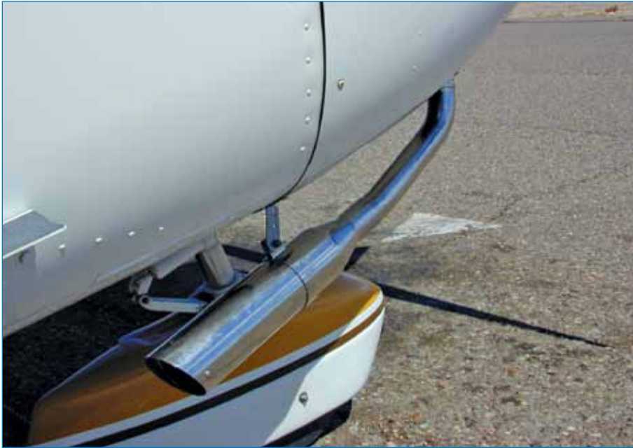
The PowerFlow exhaust mod, left, is available for many aircraft, including the PA-28-140 series.
