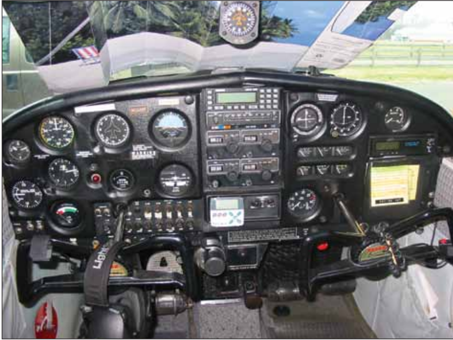
By modern standards, PA-28-140 panels are rudimentary but nonetheless perfectly functional. Pete Hodges' 1969 140 still has the original Bendix/King KX-170 navcomms and the non-standard instrument layout popular in aircraft of the era.
