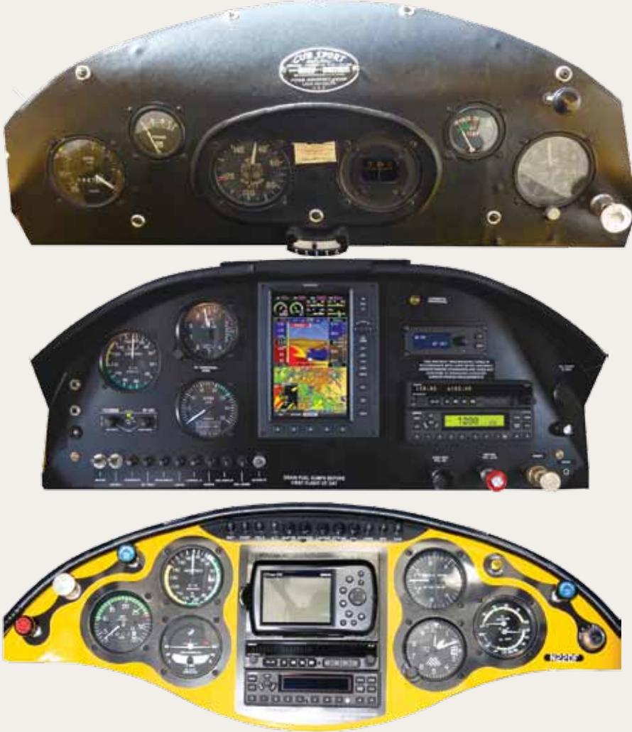
A J-3's panel, top, is 1930s minimalist. But for both the Legend, (center) and the Sport Cub, avionics choices are considerable, ranging from Garmin portables to Dynon's top-of-the-line EFIS units. The Sport Cub's design (lower) tends toward the more colorful and stylish.
