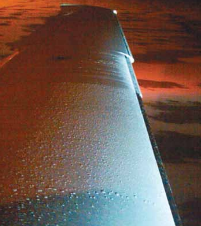
That's ice on the wing of this FIKI Cirrus after landing. Moderate icing may not entirely clear. (Photo: Bill Straw)
