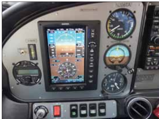
The P2008's panel is big-airplane like, with a single Garmin G3X, a center stack and analog engine instruments to the far right. Fuel switch is plainly in view at the bottom of the stack, lower photo.
