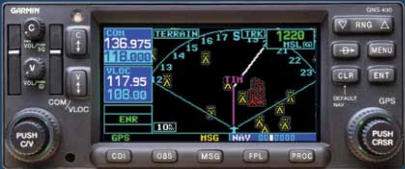
Image above illustrates how Garmin squeezed more screen real estate out of the same size box. GTN650, above, is 53 percent larger than the GNS430, below. Elimination of 12 of the 430's 16 keys and knobs helped. Most functions begin with the hard home key in upper right.
