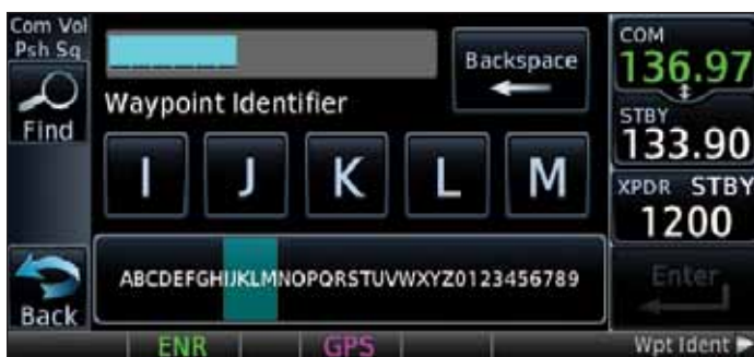
Images above illustrate how the two navigators display the keyboard. The GTN750, top, presents a full A-Z virtual pad while the GTN650, lower, uses a horizontal slider tape with a zone locator sub-tape below.
