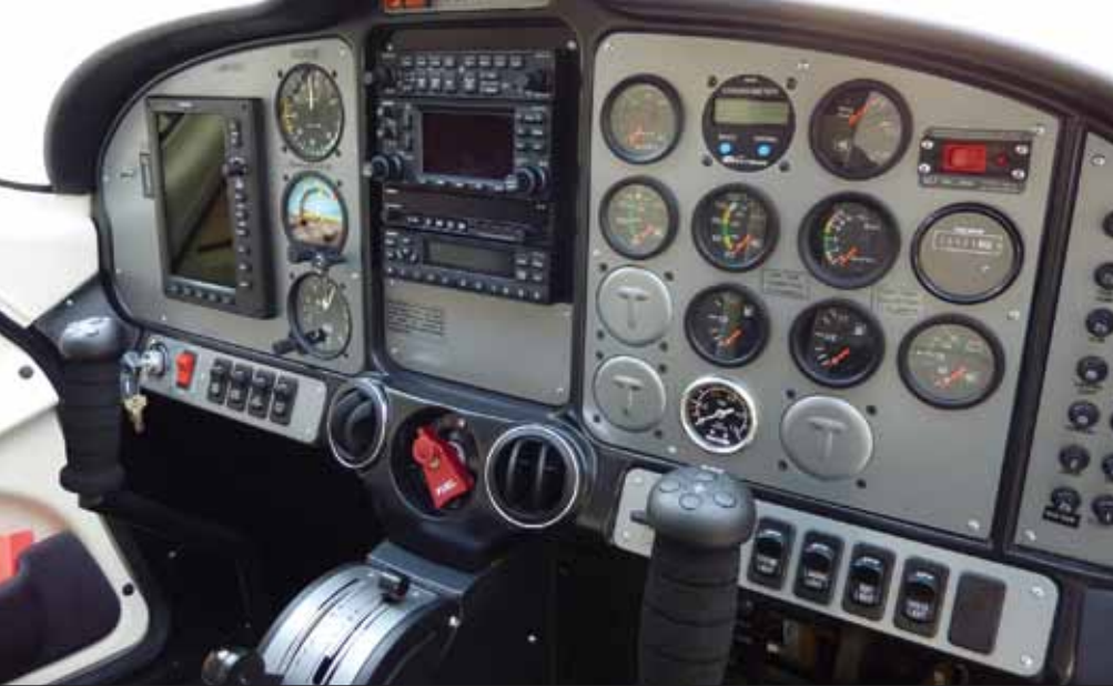
The P2008's panel is big-airplane like, with a single Garmin G3X, a center stack and analog engine instruments to the far right. Fuel switch is plainly in view at the bottom of the stack, lower photo.
