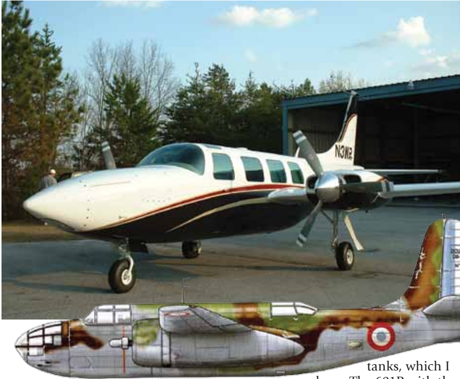
Bob Davis sent us the top photo of a 600, whose characteristic mid-wing was a Ted Smith signature design feature. He used it on the Douglas A-20 Havoc attack bomber, lower, known as the Boston by the RAF.
