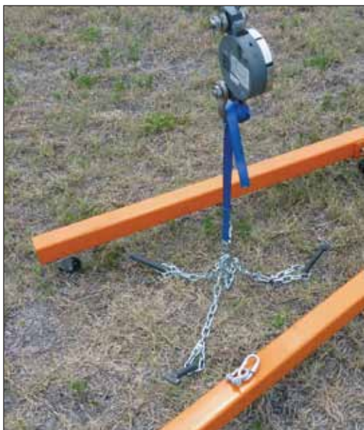
Top photo, the shopmade pin system, Abe's tiedown and the Storm Force were all tested in the same soil, using an engine hoist, left. Measurements were done with a Dillon mechanical dynamometer.
