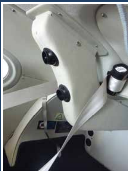
Premier's AC installation puts the compressor on the lower front of the engine, left, requiring a squarish bump in the cowl, lower left. Condenser air intake, upper left, is always open, imparting some drag. Photo above shows plenum and eye-ball vents for rear passengers.
