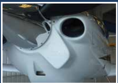
Premier's AC installation puts the compressor on the lower front of the engine, left, requiring a squarish bump in the cowl, lower left. Condenser air intake, upper left, is always open, imparting some drag. Photo above shows plenum and eye-ball vents for rear passengers.
