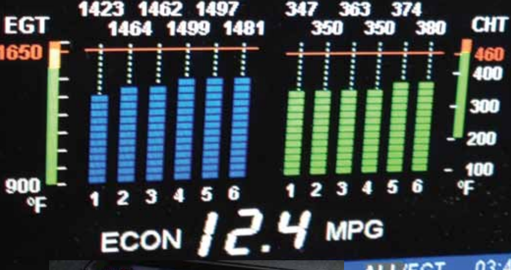
A panel shot during lean of peak cruise (inset, left), showing head temperatures at or below 380 degrees. Full shot of engine monitor (lower left) shows all operating parameters.
