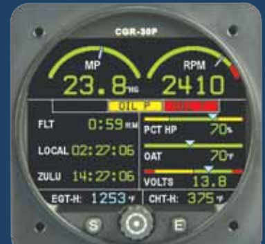
The secondary screen, above, announces main page alerts while displaying six additional engine monitoring functions.
