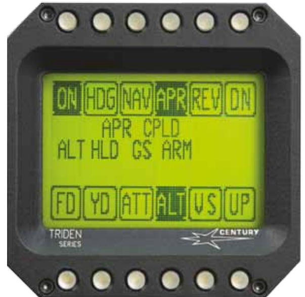
The Century 4000, top photo, and the Century Triden autopilot, middle, differ by the mounting configuration of the control head. The S-Tec 30 integrated autopilot and turn coordinator, bottom photo, saves the most panel space.
