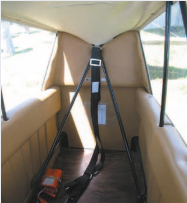
Retrofit shoulder harness in an Aeronca Champ installed as a minor modification (logbook entry only) per AC 23-17C.
