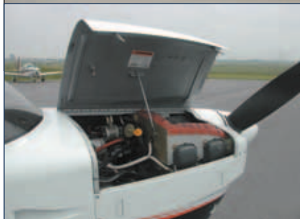
During taxi, top photo, the Tiger's castering nosewheel can play with your emotions. Lycoming's parallel valve 180-HP O-360, bottom, is easy to access under a hinged split-cowling.
