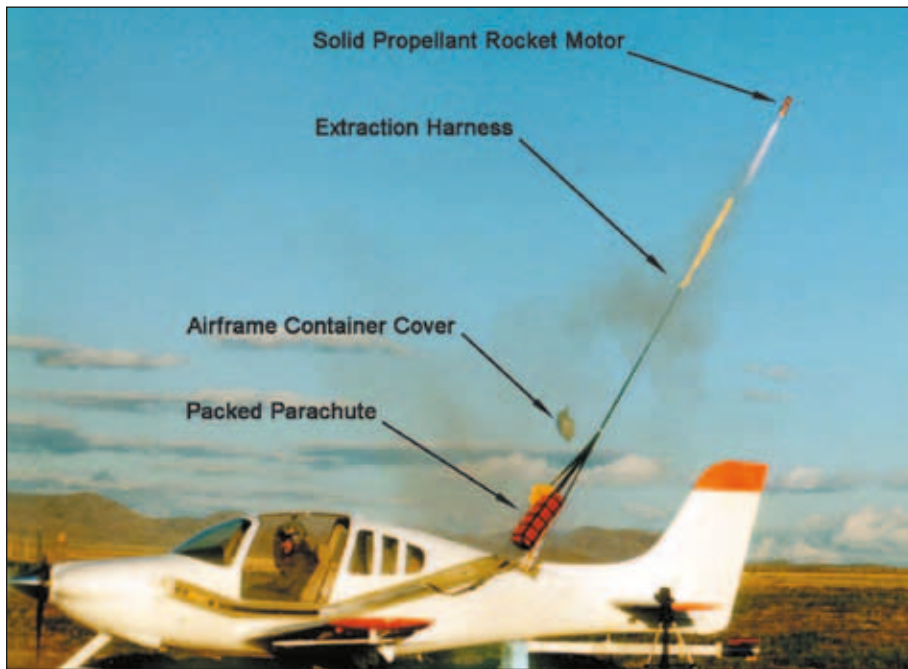
Ballistic Recovery Systems whole-airplane parachute components, left. AmSafe airbag restraint system components laid out ready for installation, lower left.
