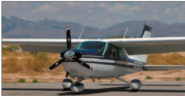
A three-blade prop looks sexy, but some owners say it's extra drag and weight on the Cardinal's nose.
