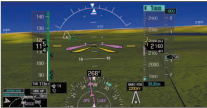
Clockwise from lower left: EVS is perhaps most useful on approach, adding another layer of awareness to synthetic vision software. If the sensor picks up the lead-in lights before nearing minimums, your eyes should soon follow.
