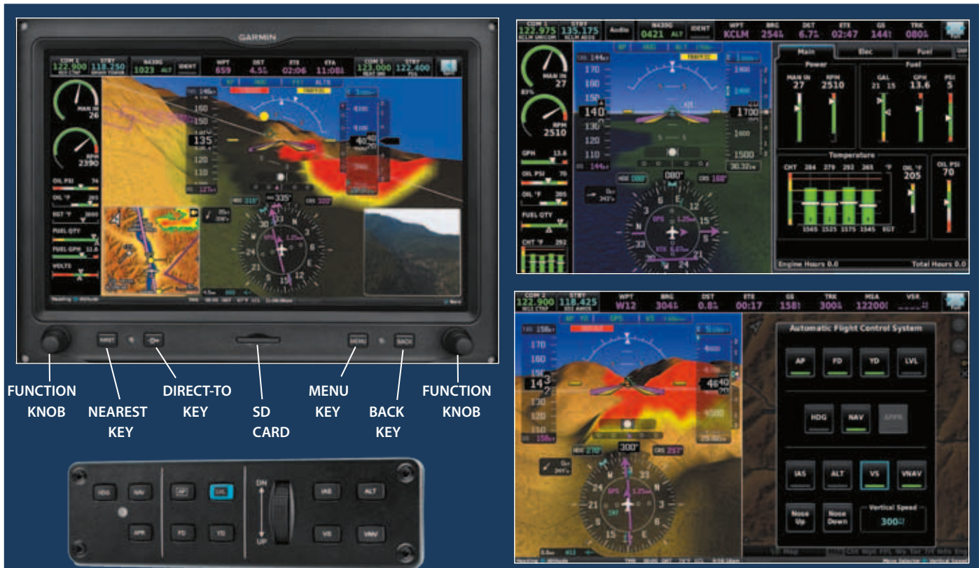
Clockwise from upper left: The GDU46X display primarily uses a touchscreen user interface, but four dedicated bezel keys and two rotary function knobs supplement some of the onscreen commands. Engine instrumentation—via the EIS engine instrumentation module—can be displayed in a split-screen view with the PFD. There’s an optional lean assist mode that works in conjunction with a fuel totalizer. The integral digital flight control/autopilot system can be commanded directly from a dedicated page on the MFD and with the GMC305 external autopilot control console.
