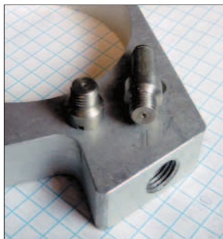
ADI fluid is stored in a five-gallon, baggage compartment-mounted tank, top photo. Fluid flows at 6 GPH through two nozzles mounted in an induction circuit plate, lower photo.
