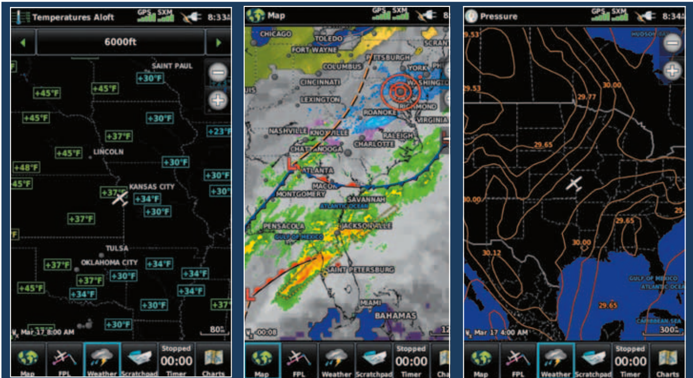
These are screen grabs of a Garmin aera796 displaying SiriusXM weather from the GXM42. From left to right: Temperatures aloft are standard in the Pilot Express package, and the aera796 feature set enables you to select temperatures for a desired altitude. Nexrad images and frontal boundaries can be displayed on a dedicated weather map page or overlaid on the navigation map. The surface pressure feature displays isobar and pressure centers on a dedicated page.
