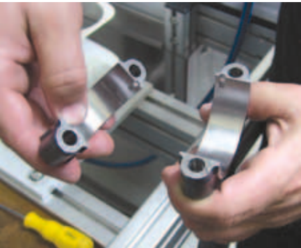
The St. Egidien factory has extensive inhouse machining capability, top, although pistons are outsourced, center. The Centurion uses automotive style "cracked" connecting rods.
