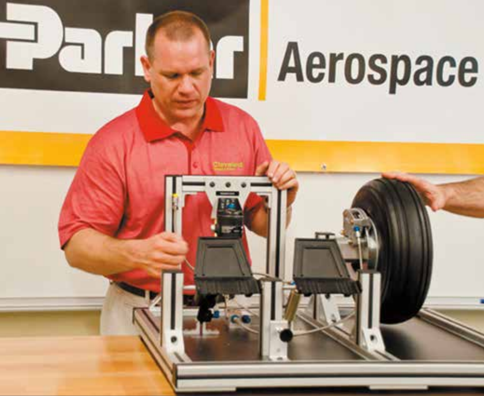
That's the Parker/Cleveland brake system training equipment, left. Typical general aviation brake system drawing courtesy of Grove Aircraft, bottom.
