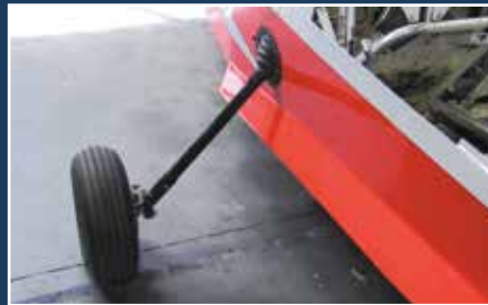
The Elite's basic hull, right, is carbon fiber and has only two through-hull fittings for the steel-tube landing gear legs, lower left. Top-side structure is built around a robust aluminum tube with bolted tubular struts, top left. Fuel tank is just aft of seats.
