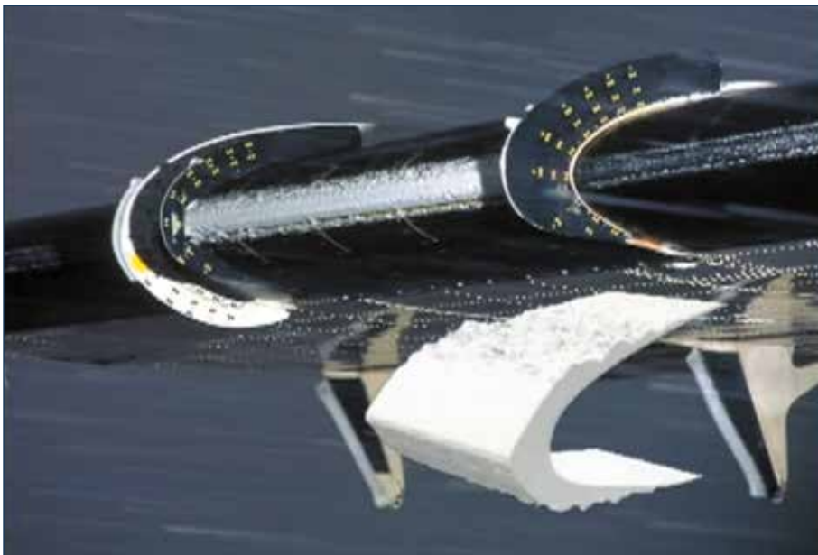
Screenshot from NASA's online course, A Pilot's Guide to In-Flight Icing, showing ice accumulation on a Twin Otter wing.
