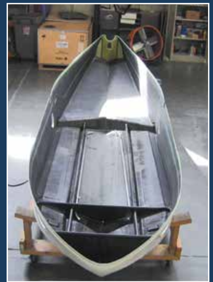
The Elite's basic hull, right, is carbon fiber and has only two through-hull fittings for the steel-tube landing gear legs, lower left. Top-side structure is built around a robust aluminum tube with bolted tubular struts, top left. Fuel tank is just aft of seats.
