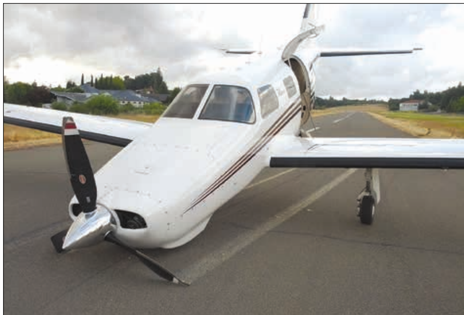
The nose landing gear has been an ongoing trouble spot for the PA-46 series. The one in the photo above has suffered a certain indignity.
