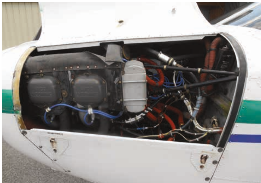
Upper cowling halves open wide, providing excellent, rapid access to engine and accessories.
