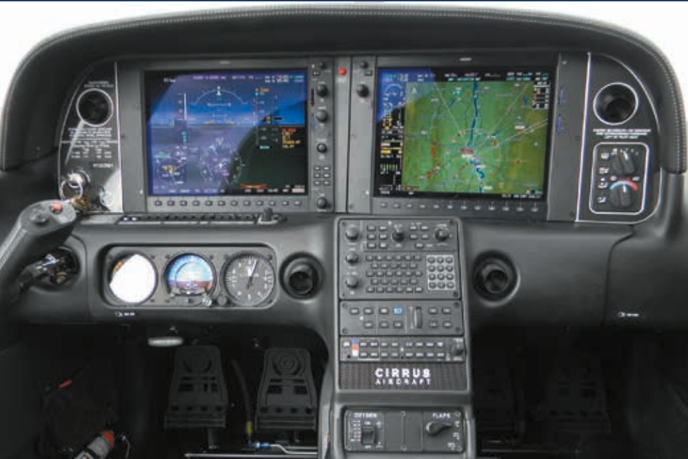
The Garmin Perspective avionics suite, top, was first offered in G3 models, replacing the Avidyne Entegra, middle. Panels in first-gen SR22s sported a combination of glass and steam gauges, bottom.
