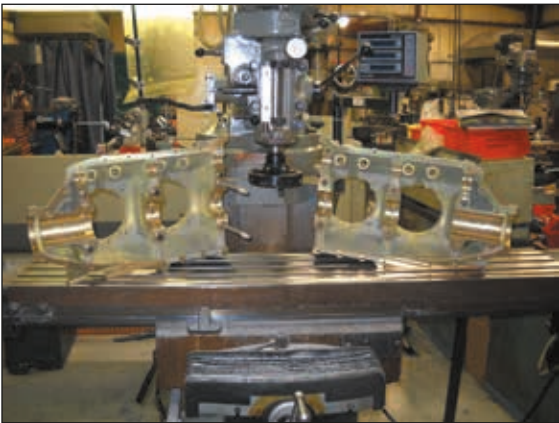
Typical crack in a large-displacement Continental case, top. It's unrepairable. As part of case overhaul, mating surfaces are cleaned up and trued, lower photo.
