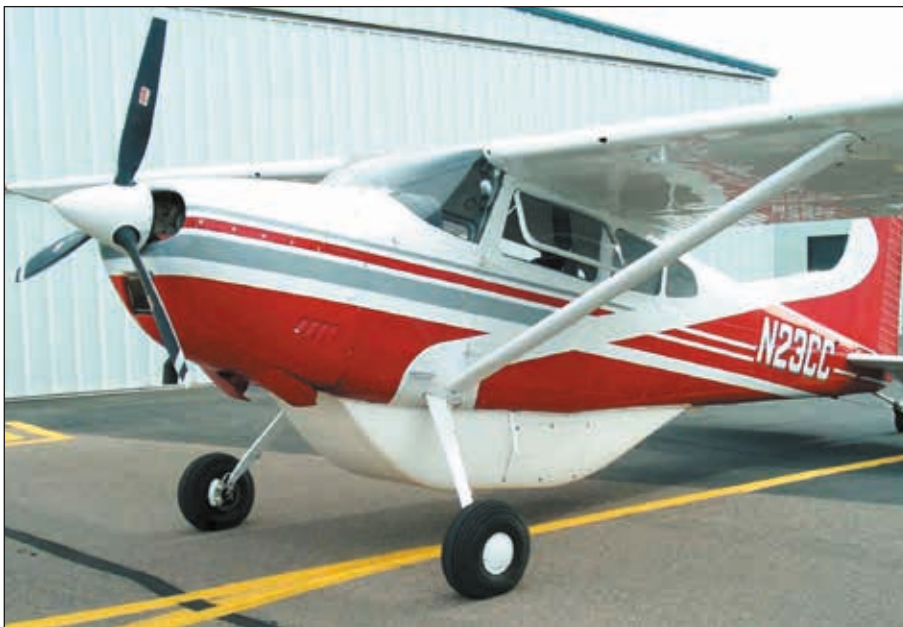
Wipaire's IO-550 engine kit is a popular mod for the 185. That's a belly cargo pod installed on the 185 in the bottom photo.
