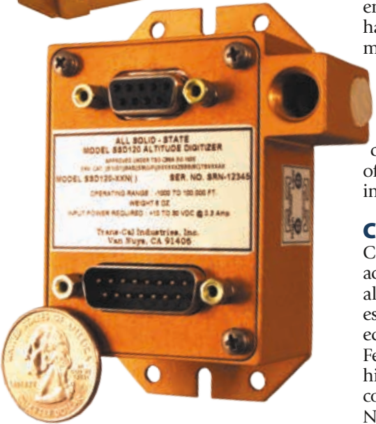
Trans-Cal's newest product is the C or "Charlie" series above. It's meant to be a lower-price option with the same basic capabilities as Trans-Cal's established Nano line, center. Increasingly, the encoder function is being displaced by air data computers like the Sandia SAC 7-35, below. Even legacy aircraft with glass panel upgrades may have ADCs.
