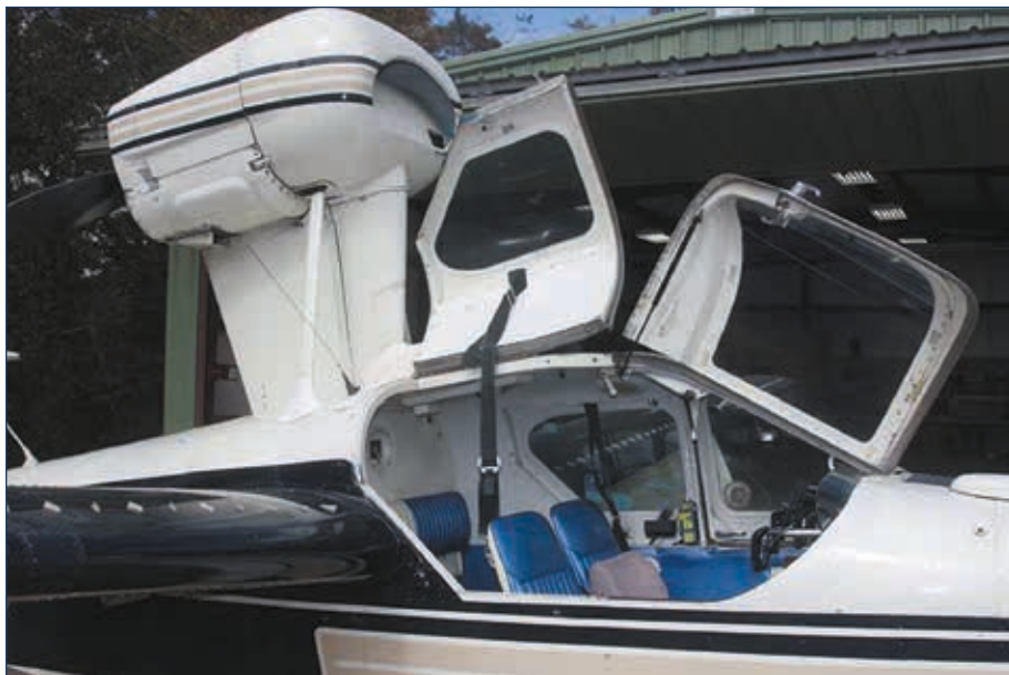
Later-model Lakes are equipped with a cargo door (above), which greatly improved cabin access. It can be retrofitted.
