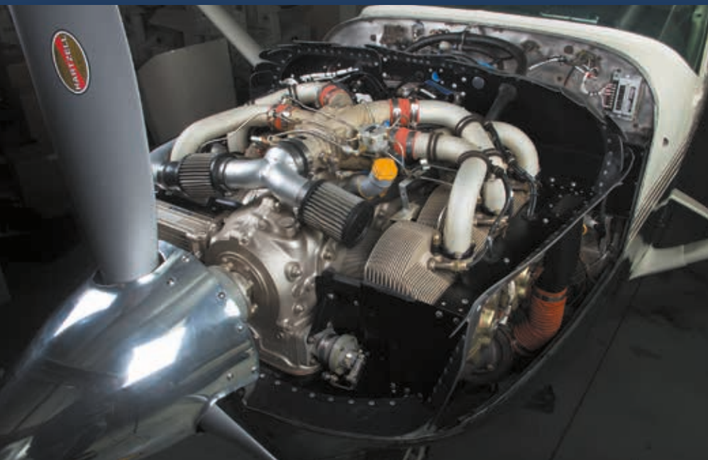
That's a Vitae 520 crossflow engine mod in the top photo. The TKS de-ice mod protects the struts, wings and elevator leading edges, middle photo. A 206 has plenty of authority on Wipaire amphibious floats, bottom.
