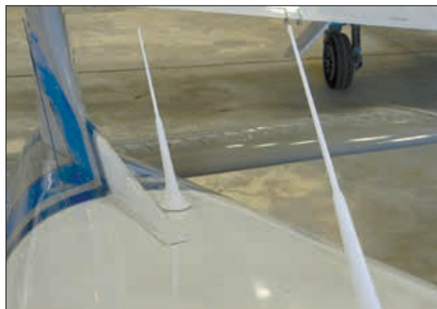
The newer Cub in the top photo has a limited ground plane for antennas on each side of the skylight. Those are replacement all-fiberglass comm antennas on the Piper in the bottom photo.
