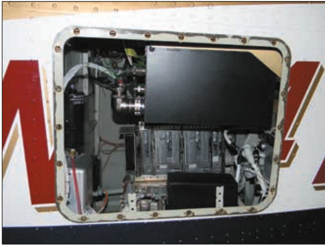
Aircraft vibration takes a toll on remote avionics that are along for the ride. The Garmin LRUs and Skywatch traffic processor in the Mooney's avionics bay, top photo, are perhaps more tolerant of long-term vibration than the Century NSD360A mechanical gyro, bottom.
