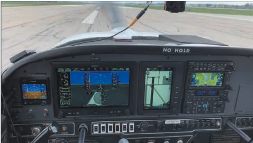
The G3X Touch at Grumman Tiger rotation speed. The PFD (middle) has integrated angle of attack, SVT synthetic vision, plus engine instruments and fuel data. This optional system is movable from the PFD to the MFD, in various screen configurations. That's split-screen EIS and map, bottom photo.
