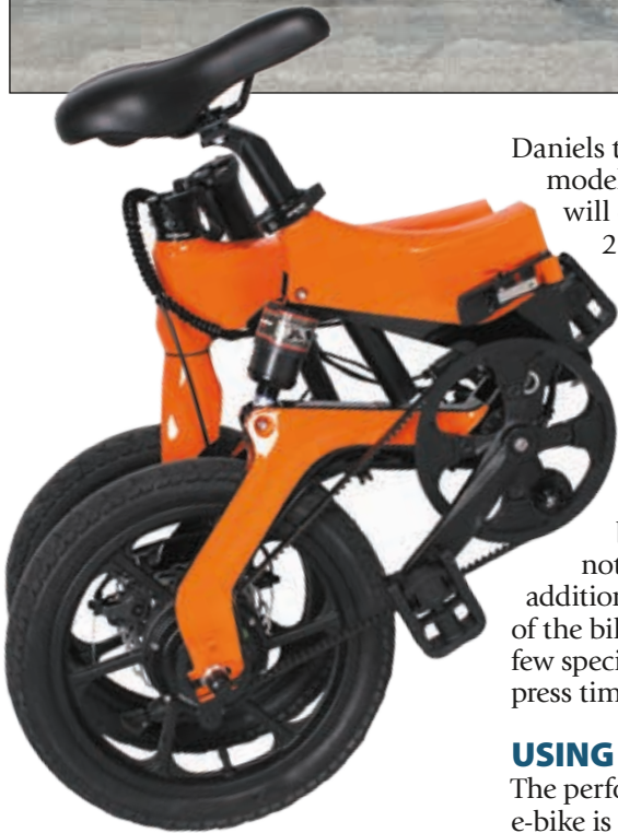
That's the Jupiter Discovery, opened and folded, in both images above. It weighs just over 42 pounds with the frame-mounted battery.
