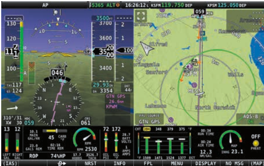
The system has screen recording and that's a capture in cruise flight. Notice the logical layout of engine data.
