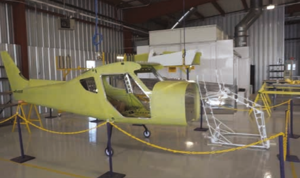
The Colt fuselage has a welded-steel cage attached to a conventional riveted monocoque tail section, left. The aircraft's standard equipment includes a ballistic parachute stored in a box behind the baggage compartment, lower photo.
