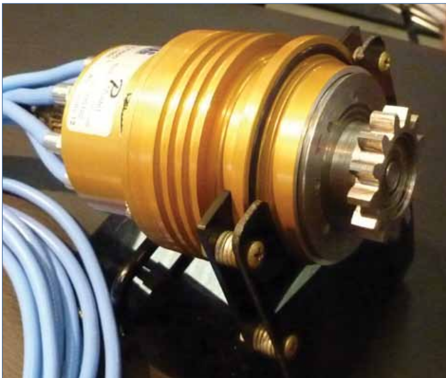
E-mag's new 200 series, above, is a clever hybrid with its own internal alternator to make low voltage. Electronic circuitry turns that into high tension for the plugs. There's a single moving part, left, a shaft with a gear.
